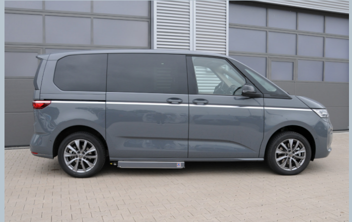
The ultra-slim K70 cassette lift combined with the vehicle heightening offers the best possible ground clearance.
