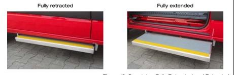
Figure 12: Smartstep Fully Retracted and Extended
