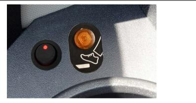
Figure 11: Deactivation Switch next to the Indicator Lamp
