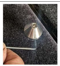
Loosening the clamping screw
