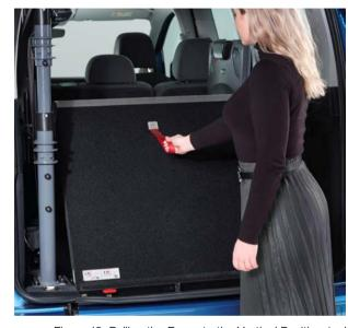
Figure 12: Pulling the Ramp to the Vertical Position (only for EasyFlex)
