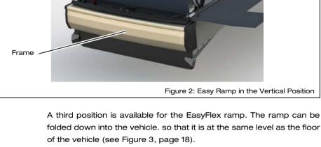
folded down into the vehicle. so that it is at the same level as the floor
