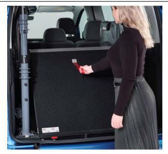
Figure 24: Stowing the Ramp
