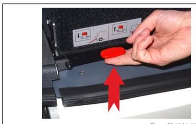
Figure 23: Unlatching the Ramp
