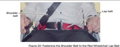
Figure 20: Fastening the Shoulder Belt to the Red Wheelchair Lap Belt
