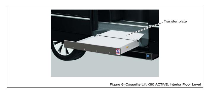
Guards are provided on all other sides of the platform to prevent the wheelchair from rolling off the platform (see Figure 5, page 15, and Figure 6).
