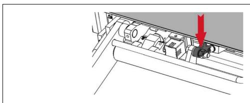
Figure 41: Adjusting the Switching Cam, View from Above (K70)
