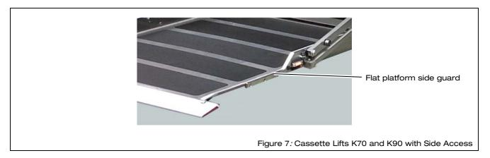
When the platform on the K70 or K90 is retracted into the cassette, the raised roll-off guard acts as a cover for the cassette (see Figure 8, page 17). With the K90 ACTIVE, the platform side guard acts as a cover for the cassette (see Figure 9, page 17). In each case this prevents dirt from entering the mechanics of the Cassette Lift.
