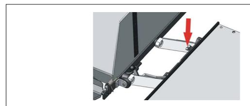
Figure 48: Adjusting the Switching Cam for the Retract Position (2)
