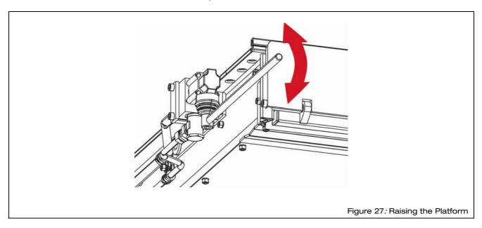
⇒ Remove the pump lever from the manually-operated pump once the platform has been raised in the emergency mode.
