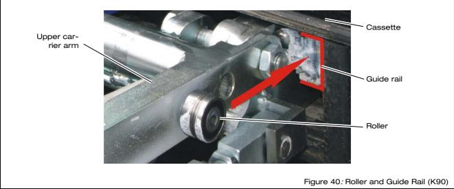
Rollers and guide rails ensure that the platform is guided precisely when being retracted into the cassette.
