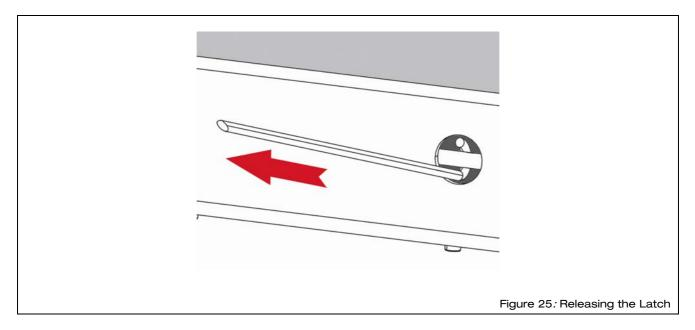
Releasing the latch releases the platform.
