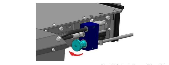
Figure 34: Closing the Pressure Release Valve
