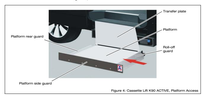
All platforms are provided with a roll-off guard that automatically rises when the platform is raised off the ground. This prevents the wheel-chair from rolling backwards off the platform.
