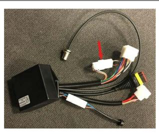
Figure 30: Control Unit and Connections for K70/ K70 / K90 ACTIVE (2)
