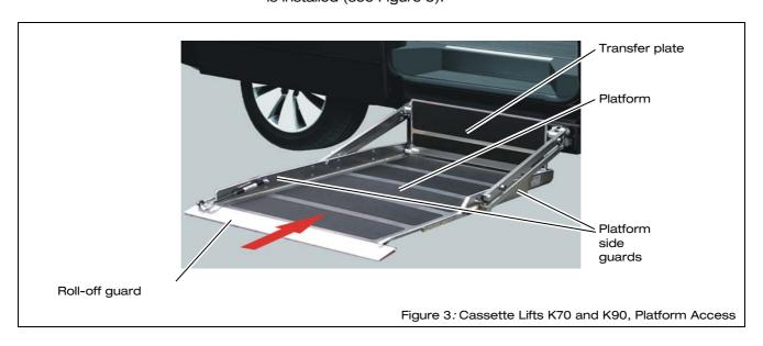
With the K90 ACTIVE, the wheelchair is pushed onto the platform parallel to the vehicle, in the direction of the rear of the vehicle (see Figure 4).
