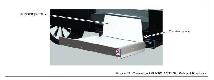
The platform is extended and retracted electrically.
