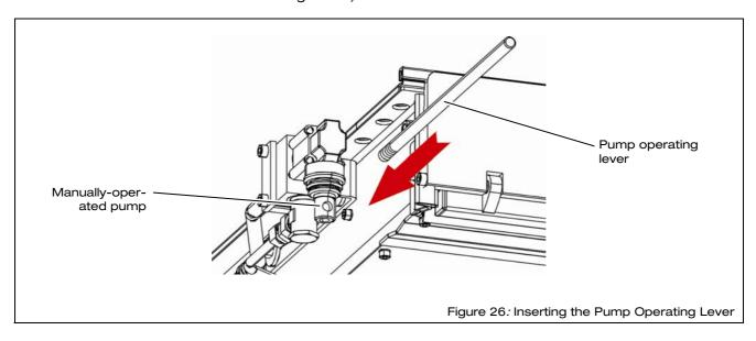
⇒ Raise the platform by pumping the pump operating lever (see Figure 27).
