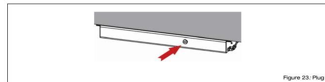
⇒ Remove the plug. To do this, use the hook provided as an accessory (see Figure 24).
