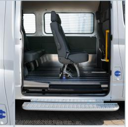
Step and grab handle at the side entry allow easy access to the passenger cabin.
