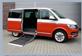
K90 in lowest position at the ground. Barrier folded down.
