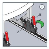
3. The handles (B) fix the seat in its new position. The security bolts (A) have to be in lowered position. Please repeat this procedure with the other seat leg to fix the seat.
