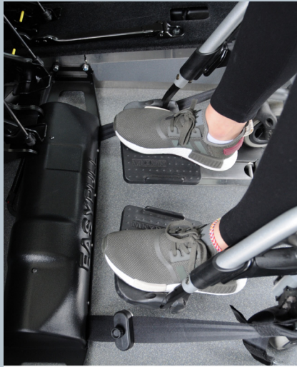
Fully integrated restraint system tested acc. ISO 10542
